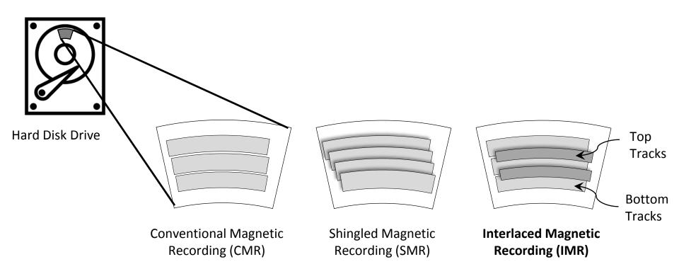
IMR: Higher areal data density than CMR, lower write amplification (WA) than SMR.
